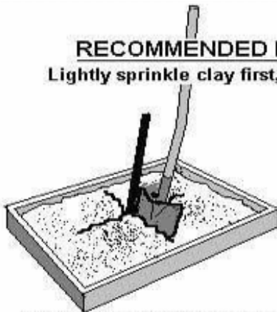
STEP 1 Hold shovel blade vertical and step on blade to make 4 cuts as shown above. Use more cuts for large pits.
